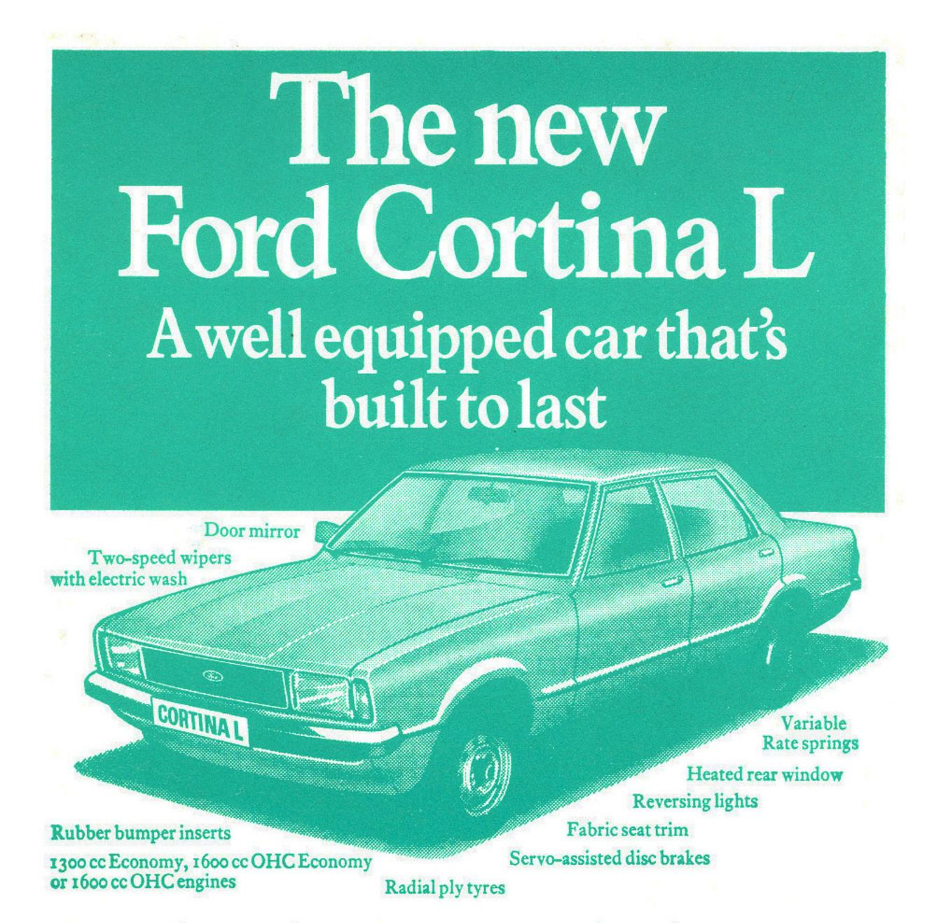
The new Ford Cortina L has more built-in equipment than ever. But even more important today, it's a thoroughly well-engineered car with features like Variable Rate rear coil springs that improve the ride and handling, the advanced Sonic Idle carburettor that contributes to economy, and the tough acrylic paint finish for good looks and durability.
